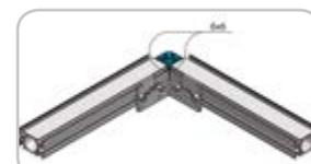
4.5. **Expansion of the line:** for lines with a straight section longer than 50 meters, we suggest mounting a sliding joint every 30 to 40 meters. This will make any future dismantling easier. The two fixing plates have to be assembled in the middle of the available space.
