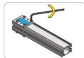
4.3. **How to tighten the screws:** The screws must be tightened but be careful not to tear the thread. The torque of the m6 screws should be between a minimum of 10 N·m (91 inch-lbs) and a maximum of 13.5 N·m (120 inch-lbs).
