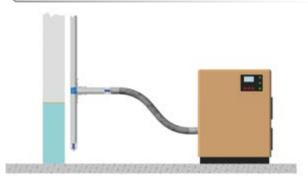
We recommend that the compressor is connected with a flexible pipe to absorb the vibrations due to the machine on every installation.
